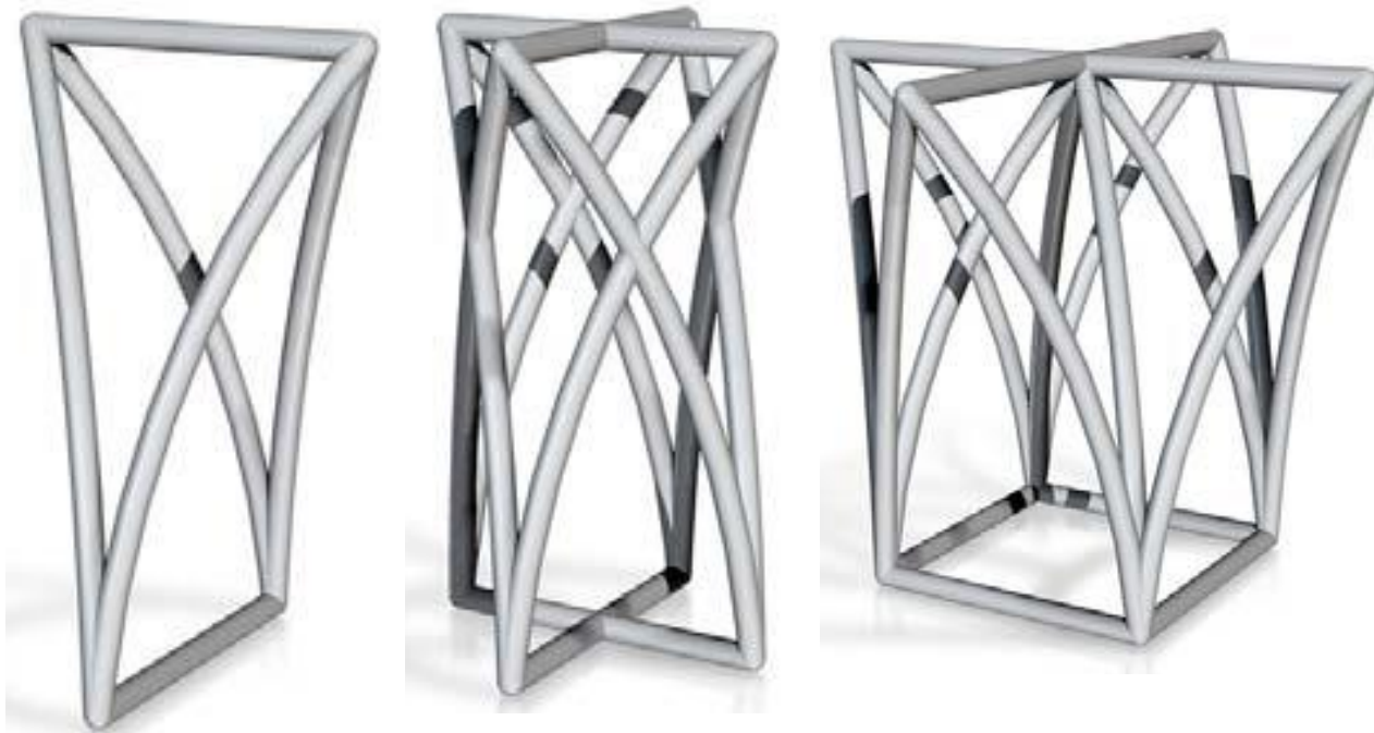
Figure 30. (a) Curve-linear Tetrahedron 5 with four cylindrical faces. (b) Quarter turn rotation of (a) joined with(a). (c) Group corresponding to (a).
