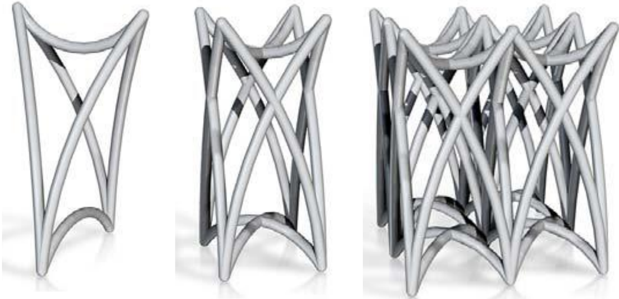
Figure 31. (a) Curved Tetrahedron 3 with four hyperbolic faces. (b) Quarter turn rotation of (a) joined with (a). (c) Group corresponding to (a).
