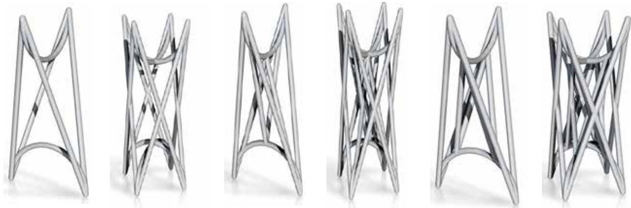
Figure 2. Figure 3. Figure 4. Figure 5. Figure 6. Figure 7. Figure 2-7. Curve-linear tetrahedron 1 with four conical faces and five variations.
