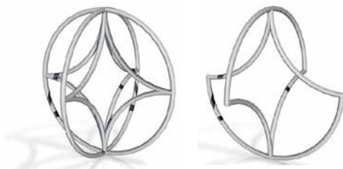
Figure 17. Femisphere as curved tetrahedron 1 with four hyperbolic faces. (a) Two femispheres (b) one femisphere
